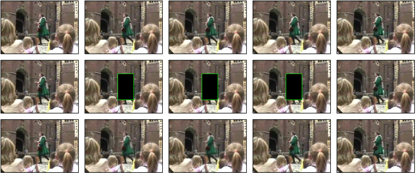
Figure 5. Performer video result (five frames shown). Top row: original image sequence, middle row: corresponding image sequence with a hole, and bottom row: result of video completion using our method.
