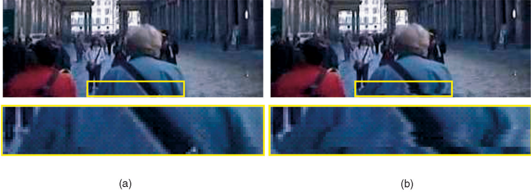
Fig. 10. Comparison of completion results. (a) Our method and (b) mosaicing. The rectangular areas in the images in the top row are closed up in the bottom row.
