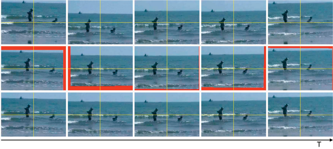
Fig. 8. Result of video stabilization #1. Top row: Original input sequence. Middle row: stabilized sequence which still has missing image areas. Bottom row: stabilized and completed sequence. The grid is overlaid for better visualization.
