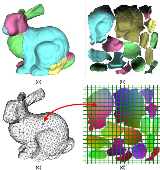
Fig. 3. Construction of a dense mesh for BTF synthesis. (a) and (b) Texture atlas. (c) and (d) Multi-chart geometry image mesh (MCGIM), which samples a surface using a regular grid. Each mesh vertex is a grid point.
