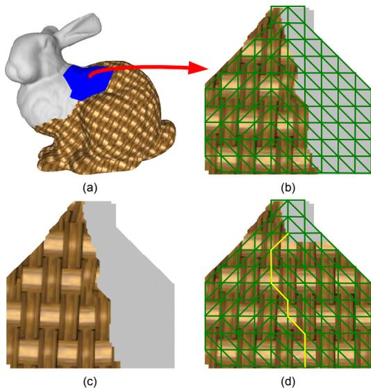
Fig. 5. BTF synthesis using a work patch and a work image. (a) Finding a work patch on the surface. (b) The initial work patch. (c) Work image with synthesized and un-synthesized pixels. (d) Work patch after fitting a new texture patch, with the graphcut seam shown in yellow.
